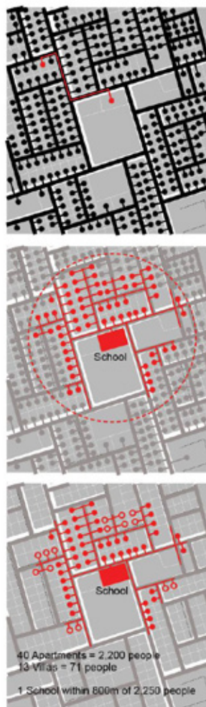
Figure 7 - Linking plots through the spatial network allowing relationships between specific plots and land uses to be calculated
