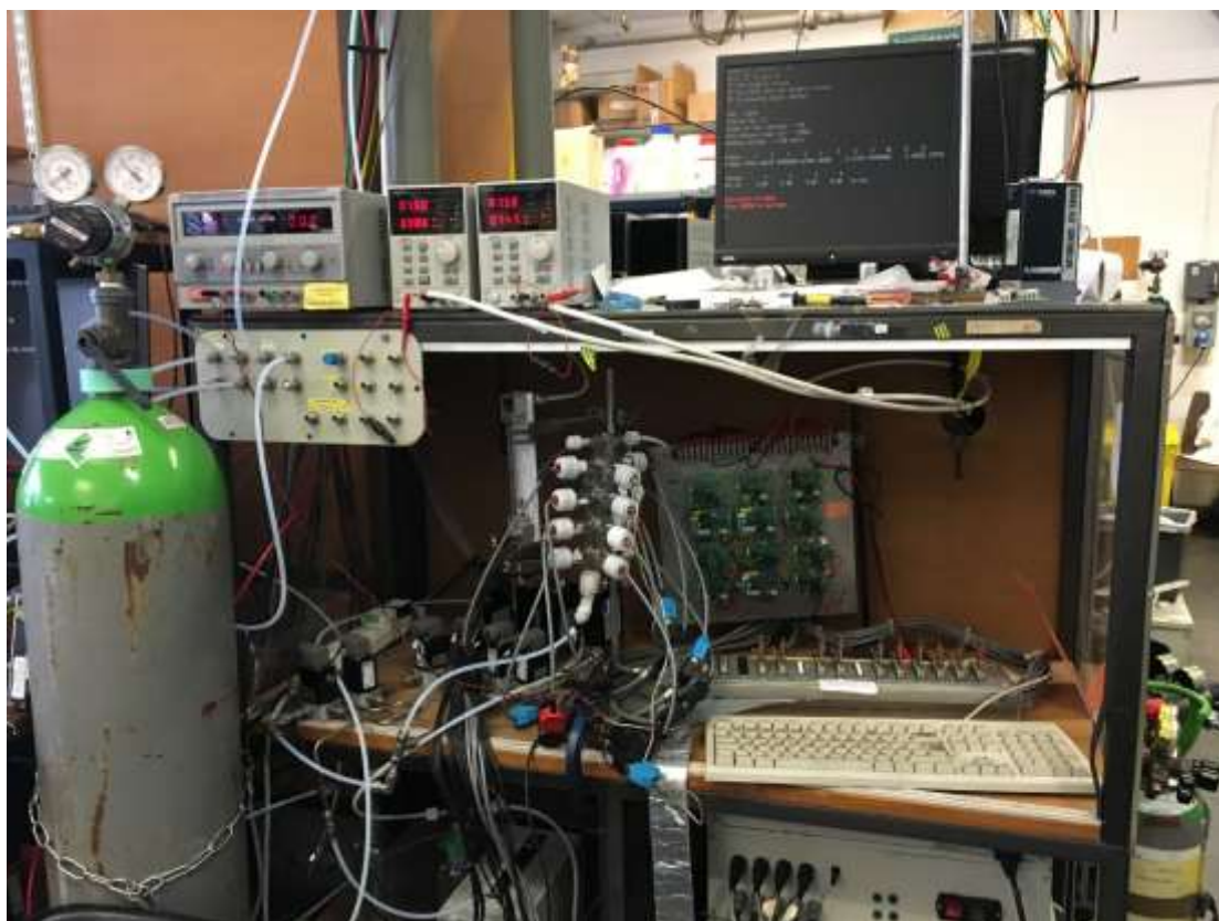
Figure 2.4. Gas sensing rig used in this investigation. The rig consists of a gas-sensing chamber, which can accommodate up to 12 ports. Gases are introduced in a controlled manner to the sensing chamber through four mass flow controllers and six solenoid valves.
