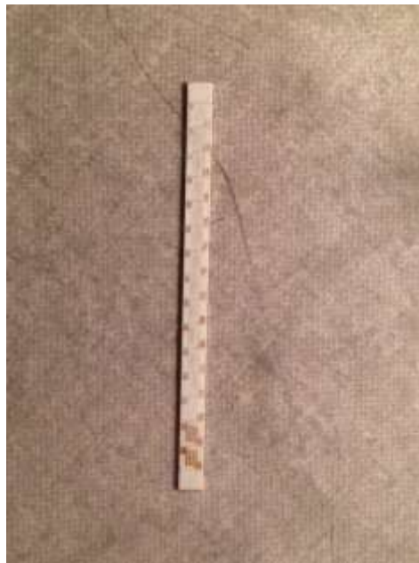
Figure 2.2. A printed strip of zinc oxide sensors.
