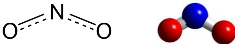
Figure 1.24. Skeletal and 3D structure of nitrogen dioxide. Nitrogen atoms are shown in blue and oxygen atoms are shown in red. The bond angle is 134.3°. Structures produced using ChemDraw (2D) and Arguslab (3D).
