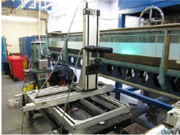
Figure 4-6: Traverse set-up with LDV
