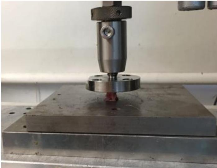
Figure 6.3: A setup to measure the compression of the L4 and L5 vertebrae. L4 and L5 vertebrae was compressed until failure to obtain a force/deformation curve using a Zwick machine.
