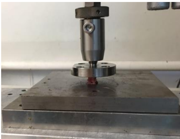
Figure 2.1: A photograph showing the compression test setup of a L4 vertebrae. L4 and L5 vertebrae was compressed until failure to obtain a force/deformation curve using a zwick machine.
