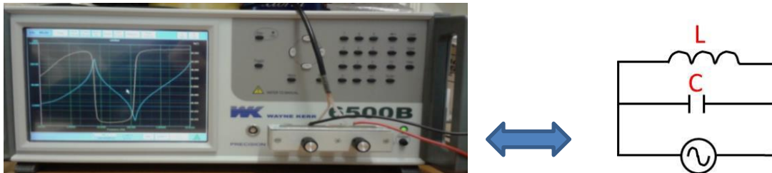
Fig. 3.2. Left: Front view of the Precision Impedance Analyzer 6500B (Wayne Kerr) used to measure the resonant frequency and Q-factor of the system, in air and in the presence of conductive samples. The display shows the resonance peak on a Z vs frequency plot. The instrument was connected to a parallel LC circuit, with electronic schematic shown on the right of the figure, which consisted in a coil (e.g. pancake coil with inductance L=970 \mu\text{H} \pm 10\% ) and a capacitor selected from the capacitor bank.
