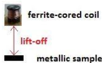
Fig. 3.6. Simplified sketch showing the experimental configuration in which a flat metallic sample was inductively coupled to an inductor (“ferrite-cored coil”) at a fixed value of lift-off, i.e., vertical distance between the sample and the ferrite-cored coil. The inductor shown here (made by “multicomp”, part no. MCSCH895-681 KU) was connected to a capacitor as shown in Figs. 3.2-3.3. This figure represents one of the two configurations used in the experiments, the second one being characterised by the LC system “in air”, i.e., with no metallic sample present.
