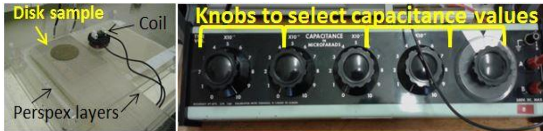
Fig. 3.1. Left: Picture of the experimental system used at the initial stage of this research work, to test whether the presence of a metallic sample could be detected by using a LCR-based system. The sample in this picture is a copper disk (6-cm-diameter, 2-mm-thickness), and the coil is a pancake coil (No. turns= 400 \pm 1 , outer diameter 43.0 \pm 0.5 mm, inner diameter 22.0 \pm 0.5 mm, height 20.0 \pm 0.5 mm). Two Perspex layers were used as a non-magnetic structure to support the coil and maintain it in a fixed position w.r.t. the sample. The coil was part of a LC circuit whose capacitance could be varied to make the system resonate at different values of resonant frequencies. This was achieved by selecting appropriate capacitance values from the “Jay-Jay instruments - Type no. VC5” capacitor bank (Educational Measurements Limited), shown in the picture on the right.
