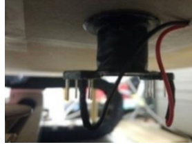
Fig. 7.20. Picture of the coil used in this study ( L=79.4\pm 10\% \mu\text{H} , height 1.8\pm 0.1 \text{ cm} , inner diameter 2.0\pm 0.1 \text{ cm} , outer diameter 2.3\pm 0.1 \text{ cm} ). The coil was connected to the other circuits' components as in Fig. 7.13.
