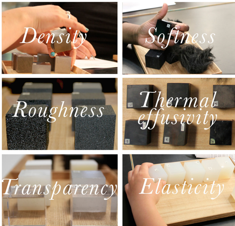
Figure 3. Photographs and property descriptors of our material collection of cubes used in the PhysFeel focus groups. Density set: tungsten, solder, cast iron, zinc, titanium and aluminium, selected for their different densities using the Cambridge Engineering Selector (CES Edupack 2016). Softness set: fake fur, fun fur, silk velvet, synthetic velvet, denim and PVC, selected for their different fibre lengths and stiffnesses. Roughness set: different grades of sandpaper from P60 to P800 grit. Thermal effusivity set: concrete, slate, vulcanized rubber, nylon, hardwood and wax, all dyed black, selected for their different thermal properties using the Cambridge Engineering Selector (CES Edupack 2016). Transparency set: plaster of Paris, nylon, polypropylene, polyurethane resin, acrylic and glass, selected for their different optical transparencies. Elasticity set: cast from silicone rubbers of different shore hardnesses (Shore 10 to 50).
