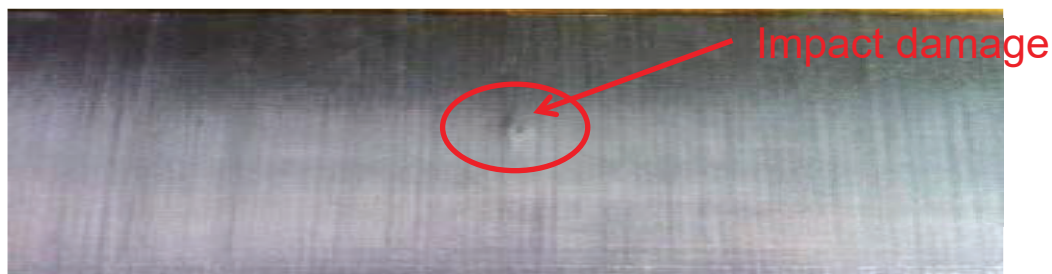
FIGURE 1. Photograph of composite specimen with barely visible impact damage marked.
