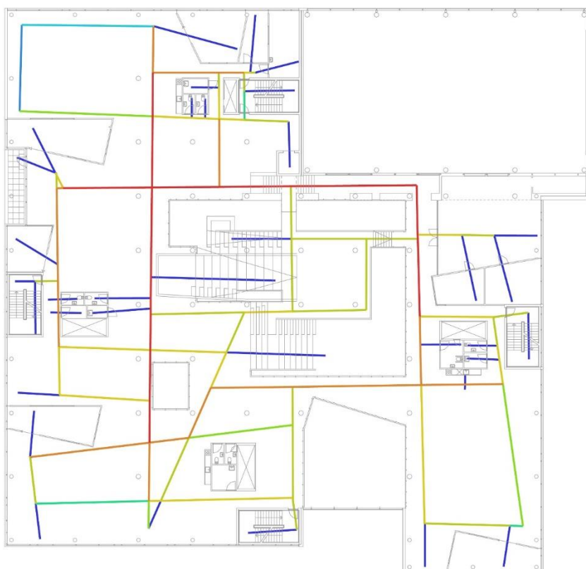
Figure 6: Floor plan of 1 st floor of Hellerup School (courtesy of Arkitema), overlaid with segment analysis showing the distribution of Normalised Angular Choice; segments in warm colours (red, orange, yellow) have higher NACH values, while segments in cooler colours (green, turquoise, blue) have lower NACH values
