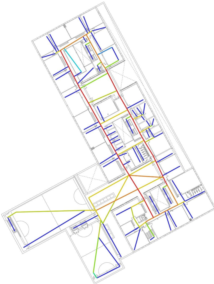
Figure 2: Floor plan of 1 st floor of Chelsea Academy (courtesy of Feilden Clegg Bradley Studios), overlaid with segment analysis showing the distribution of Normalised Angular Choice; segments in warm colours (red, orange, yellow) have higher NACH values, while segments in cooler colours (green, turquoise, blue) have lower NACH values
