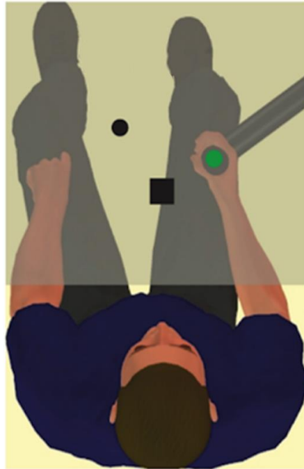
Figure 3.1 The robotic apparatus used allowed subjects to control a cursor with their hand movements. Subjects grasped a manipulandum in their semi-pronated right hand. Their view of their own arm was obscured by a screen (translucent in the diagram). The screen contained a cursor which reflected the position of the manipulandum. Targets which indicated to the subjects which movement they would have to make were displayed on the screen. Figure modified from one by J Galea.
