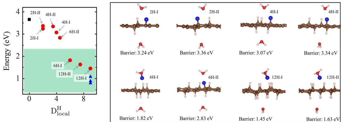
FIG. S5: cNEB barriers as a function of the local hydrogenation degree ( $D_{local}^H$ ) are shown in the left panel. The green shaded area indicates low penetration barriers with high  $D_{local}^H$ . In the right panel are the atomic structures of the initial states for the partially hydrogenated graphene as shown in the FIG S4. Red (pink, brown) balls are O (H, C) atoms. Protons are represented by blue balls.
