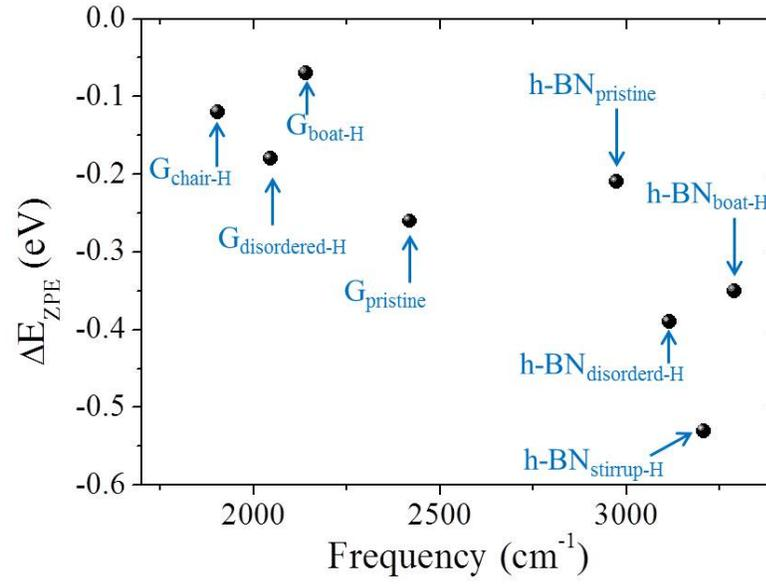
FIG. S12: The calculated ZPE correction ( $\Delta E_{\text{ZPE}}$ ) along with the stretching frequencies of the covalent bonds between proton and O, C and N atoms in the initial state of each system studied (pristine and hydrogenated 2D sheets).
