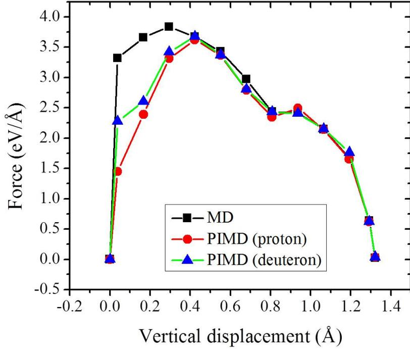
FIG. S10: The classical and quantum (proton/deuteron) constraint force profiles obtained with *ab initio* constrained MD and PIMD simulations. The standard errors of these mean forces are smaller than 90 meV/Å.
