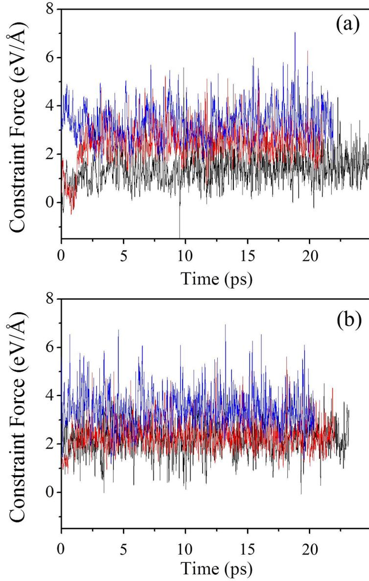
FIG. S8: The constraint forces during PIMD simulations, along with the simulation time for (a) H and (b) D nuclei, at the vertical displacement of  $0.0389 \text{ \AA}$  (black lines),  $0.1671 \text{ \AA}$  (red lines) and  $0.2953 \text{ \AA}$  (blue lines), respectively. After thermalization ( $\sim 5 \text{ ps}$ ), 30,000 steps (15 ps) were collected to calculate the constraint force, at each constraint point.
