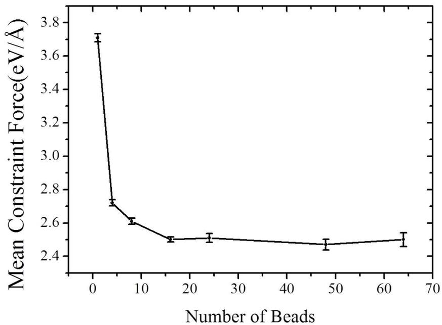
FIG. S7: The mean constraint force as a function of PIMD beads, for the proton above the graphene layer with a vertical displacement of  $0.18 \text{ \AA}$ . A vertical displacement of 0 means the plane of the graphene layer (the C atoms fixed during the PIMD simulations).
