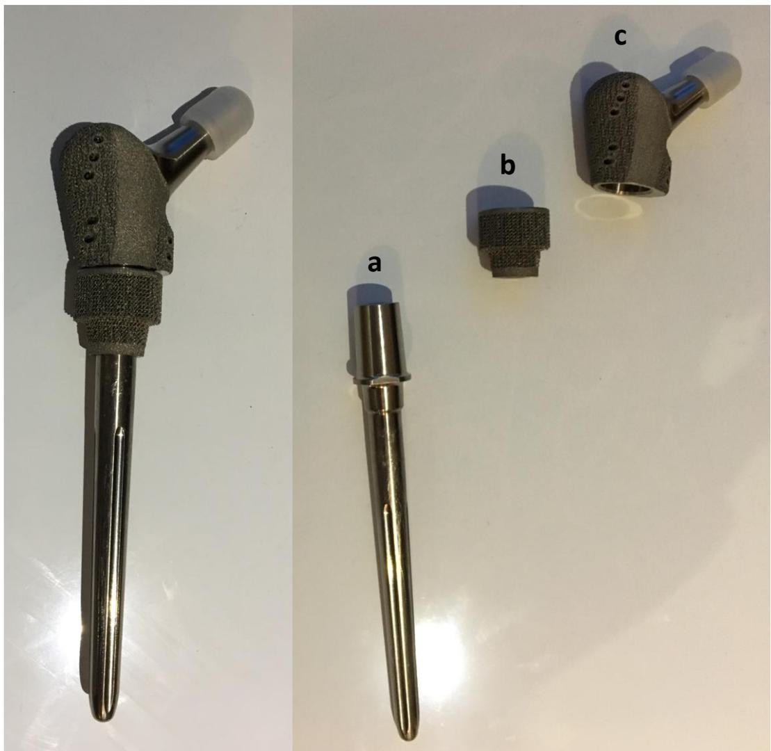
Figure 7-1 SLS Ti<sub>6</sub>Al<sub>4</sub>V proximal femoral replacement. Assembled (left) and exploded (right) implant views shown with (a) intramedullary stem, (b) ingrowth collar and (c) proximal femur with ingrowth regions for soft tissue attachments.
