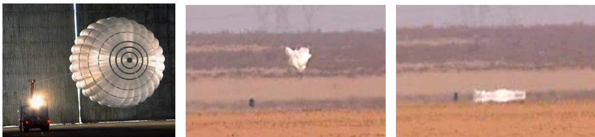
Figure 9: Main Parachute Structural Load and Drop Tests
