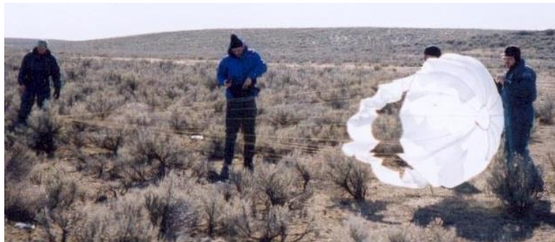
Figure 12: Pilot Parachute on test (inflated by wind)
