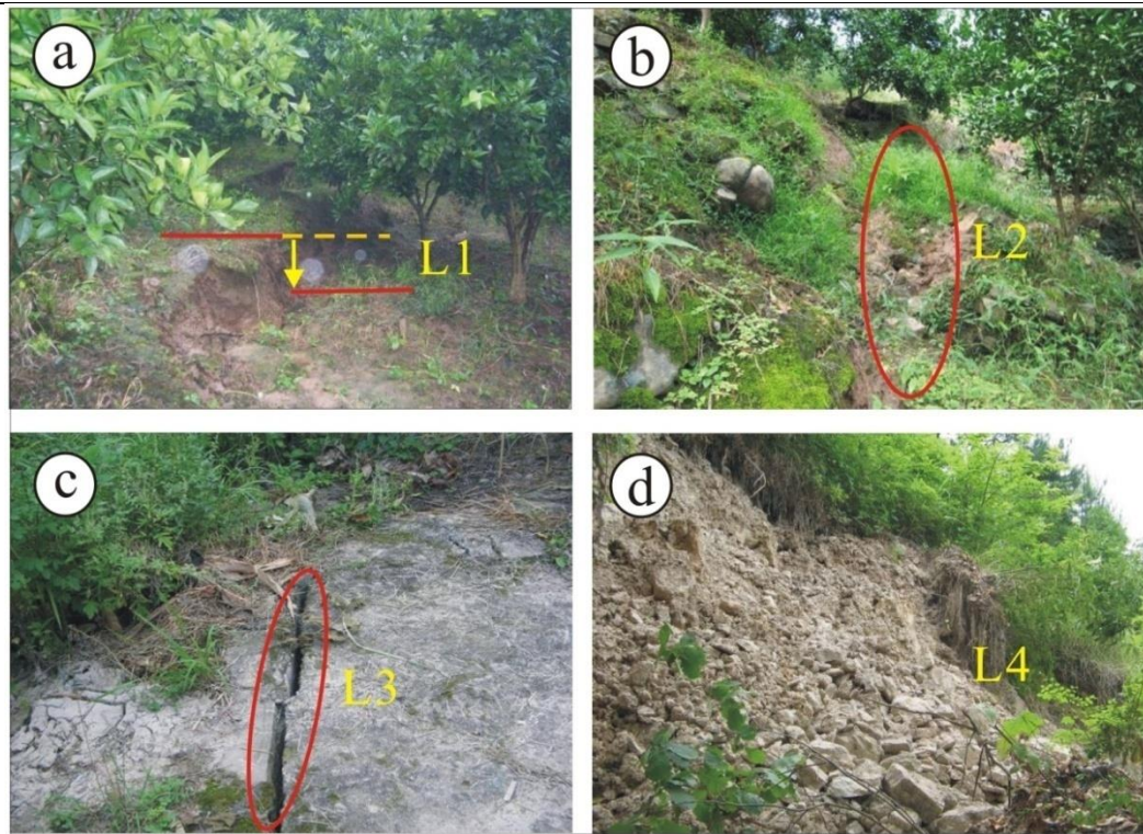
Fig. 9 Deformation indications on Baishuihe landslide
