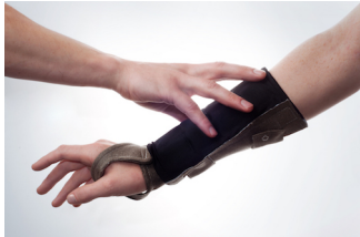
Figure 3: Wearable textile sensors can be used to detect socially relevant touches (Huisman et al., 2013).
