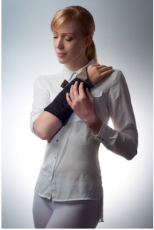
Figure 2: The Tactile Sleeve for Social Touch (TaSST) was designed to allow two individuals to engage in social touch at a distance (Huisman et al., 2013).
