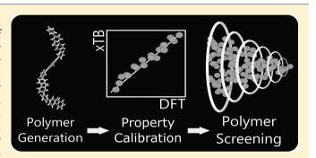
after an initial computational investment for calibration, this approach can be used to quickly and accurately screen on the order of thousands of polymers for target applications. We also demonstrate that the (opto)electronic properties of the conjugated polymers show only a very minor variation when considering different conformers and that the results of high-throughput screening are therefore expected to be relatively insensitive with respect to the conformer search methodology applied.
