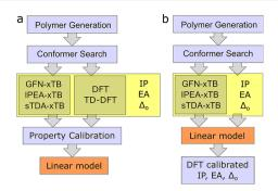
**Figure 1.** (a) Workflow of the calibration procedure, resulting in the linear model used to calibrate semiempirically determined properties (IP, EA, and optical gap ( $\Delta_o$ )) to DFT-level calculations. (b) Subsequent proposed high-throughput screening approach, where the linear model produced in panel a is applied to new polymer structures for optoelectronic property screening.
