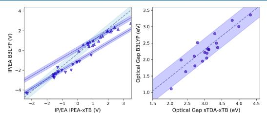
**Figure 5.** (a) IP (triangles)/EA (circles) and (b) optical gap (circles) values computed at IPEA-xTB/sTDA-xTB and B3LYP/DZP level for the validation set (Figure S3). In each case, a dielectric screening model for benzene is used. The corresponding linear regression prediction line and 95% prediction bounds from Figures 3 and 4 are included. Analogous results obtained using a dielectric screening model for water can be found in Figure S19 of the Supporting Information.
