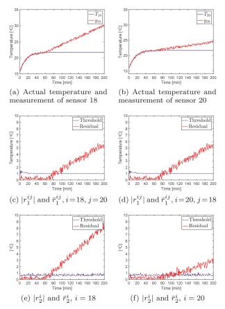
Fig. 5. Comparison between sensor 18, affected by fault  $f_{(18)}(k) = 0.06 \cdot u(k - k_{f_{18}})$  at  $k_{f_{18}} = 60$  min and sensor 20 affected by  $f_{(20)}(k) = 0.02 \cdot u(k - k_{f_{20}})$ .
