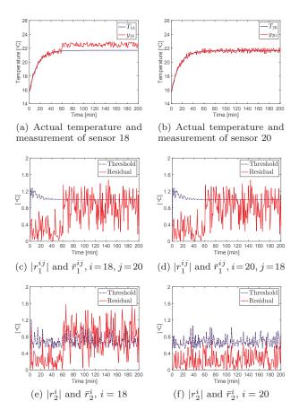
Fig. 2. Comparison between sensor 18, affected by a single sudden fault  $f_{(18)}(k) = 0.8 \cdot u(k - k_{f_{18}})$  at  $k_{f_{18}} = 60$  min, and the healthy sensor 20.
