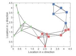
Fig. 1. IWSN with 20 sensors. The green nodes belong to  $C_1$ , the red nodes belong to  $C_2$  and the blue ones belong to  $\mathcal{C}_3$ .
