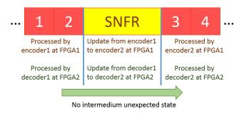
Fig. 3. The solution to synchronize the reconfiguration of coherent FPGA functions on disaggregated FPGA resources.
