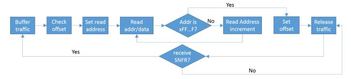
Fig. 6. The sate machine of the protocol processing unit.
