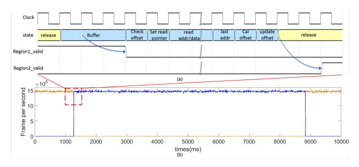
Fig. 7. The captured reconfiguration process. a) The state machine of the protocol processing unit captured by Xilinx debug core. b) The reconfiguration of output port monitored by the external traffic analyzer.
