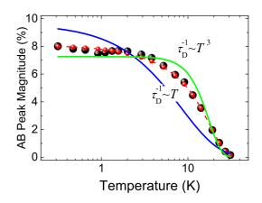
FIG. 5. Magnitude of the AB peak as a function of the temperature. The red dashed line is the fit to the functional dependence that accounts for electron-phonon and electron-electron scattering [Eq. (10)]. Solid lines (green and blue) show dependencies arising from each mechanism, separately.
