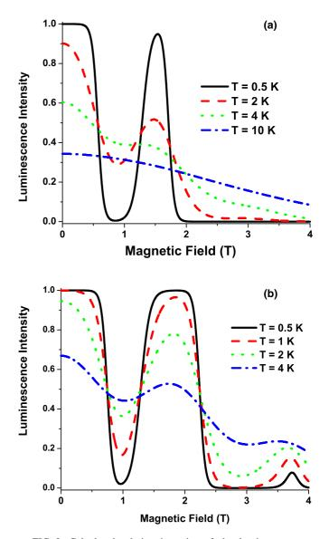
FIG. 3. Calculated relative intensity of the luminescence as a function of magnetic field for various temperatures in the case of weakly-bound excitons. (a)  $R_h = 16 \text{ nm}$ ,  $R_e = 24 \text{ nm}$ ; (b)  $R_h = 16 \text{ nm}$ ,  $R_e = 21 \text{ nm}$ .
