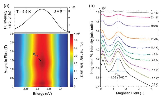
FIG. 1. (a) Photoluminescence of a sample with type-II QDs at a zero magnetic field. (b) Magneto-PL of the same sample at the same temperature with magnetic fields up to 4 T; the peak at  $\sim$ 1.38 T is due to EABE. (c) Integrated PL as a function of the magnetic field at different temperatures. Note: The plots are not shifted; rather, they show actual experimental values.
