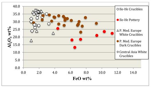
Figure 18. Comparison of alumina vs FeO content of Ile-Ife crucibles with the Ile-Ife domestic pottery and the post-medieval European crucibles (post-medieval European data from Martinón-Torres & Rehren 2009; Central Asian data from Rehren & Papachristou 2003).
