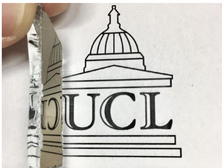
Figure 5 Photograph showing mirror-like silver film grown from silver(I) triflate on glass under nitrogen.
