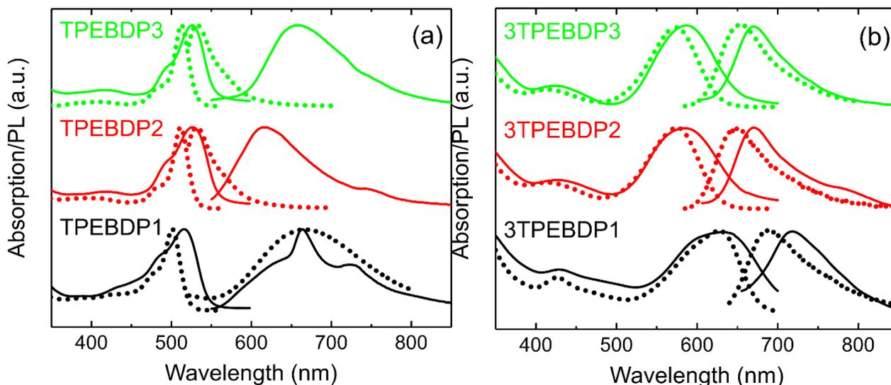
**Figure 3.** Absorption and emission of TPEBDP $x$  and 3TPEBDP $x$  in diluted THF solution (dotted lines) and solid-state thin films (full lines). For the PL experiments, samples were excited with a 520 nm laser diode (average power < 1 mW).
