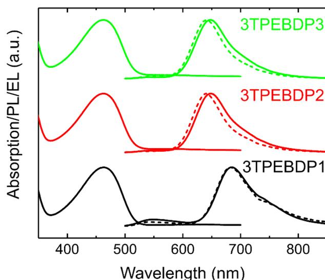
**Figure 4.** Absorption, PL and EL spectra (dashed lines) of 3TPEBDPx:F8BT blends with 1 w/w% of 3TPEBDPx loading. The absorption spectra of the blends are dominated by the F8BT band peaking at 460 nm.
