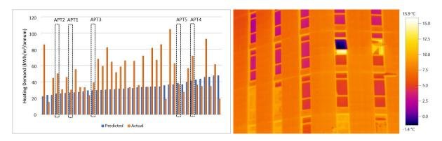
Figure 1. Actual vs. design heating demand, and external envelope thermographic survey
