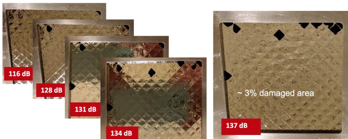
Figure 11. Pictures of the test filter sample #5, representative of a single quadrant of the LDA OBF, taken after each acoustic test performed at increasing load level with maximum SPL @ 125 Hz ranging from 116 dB to 137 dB. The last value corresponds to the Ariane 5 launch reference acoustic spectrum.
