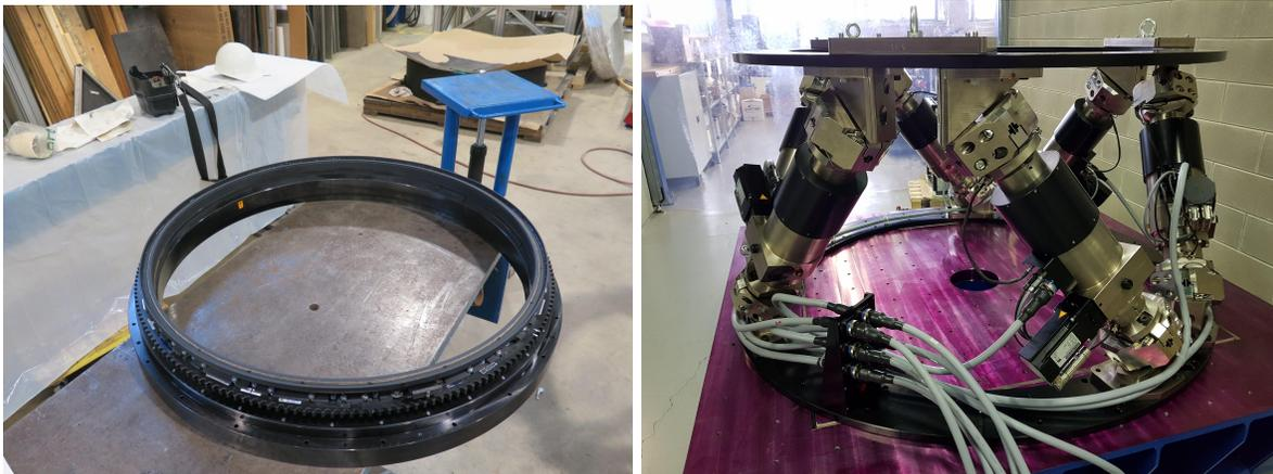
Figure 5. The picture on the left shows one of the two ADC rotator bearing and gear segments. The outer race of the bearings attaches to the Middle section and the inner race to the ADC lens cell. The gear is driven by a harmonic drive mounted to the outside of the Middle section. The picture on the right shows the final assembly of the hexapod at A.D.S International LLC.
