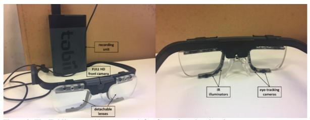
Figure 2. The Tobii eye-tracking system; left – front view showing the scene camera, detachable lenses and recoding unit; right – back view showing the eye-tracking cameras and IR illuminators
