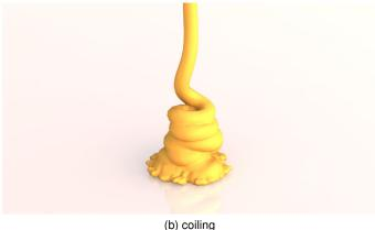
Fig. 8. Realistic buckling and coiling effects simulated with our implicit viscosity solver. Left: a sheet of 150k fluid particles is emitted with a viscosity parameter of  $\gamma=0.25$  to simulate buckling. Right: coiling is simulated by emitting 37k fluid particles with  $\gamma=0.75$ .
