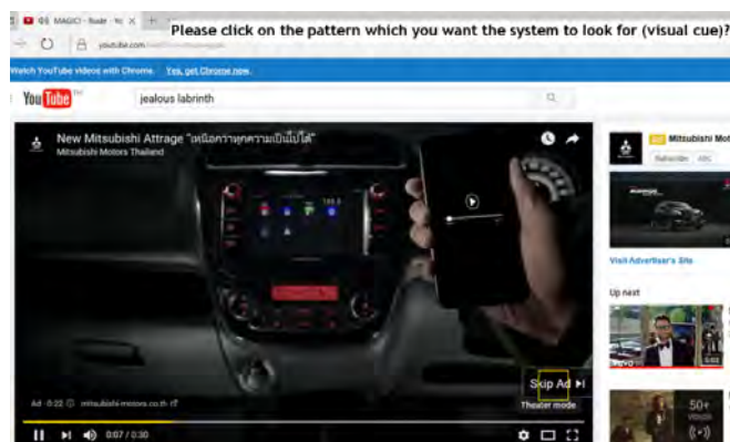
Figure 3.10: An example screenshot of HILC when it requests a user to provide the visual cue (yellow box) which is the visual pattern that invokes the system to run the rest of the script whenever the system finds it.
