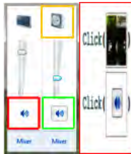
Figure 3.12: The instructor clicked on the speaker in the green box, but the system also detected a similar pattern - the speaker in the red box. In this situation, the system asks the teacher for a supporter(s), the yellow box, to help with detecting the intended pattern.
