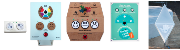
Figure 7: Iterative design process of a series of tangible interfaces: 1 - Swipe-I-Like, 2 - Smart Citizen Sentiment Dashboard, Version 01, 3 - Smart Citizen Sentiment Dashboard, Version 2, 4 - Sentiment Dashboard for the ASC installation and 5 - the Heart Rate Dashboard for the VSC; whilst 1-4 are base on RFID-card reader technology 5 has an integrated pulse sensor instead.
