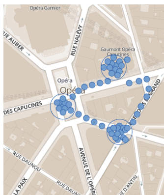
Fig. 3: Three POIs have been extracted from this mobility trace by using a clustering algorithm.
