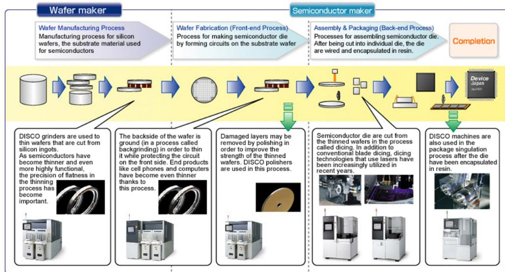
The manufacturing process of semi-conductor to help the understandings.
