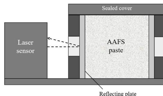
**Figure 2.** Schematic section view of autogenous shrinkage measurement.
