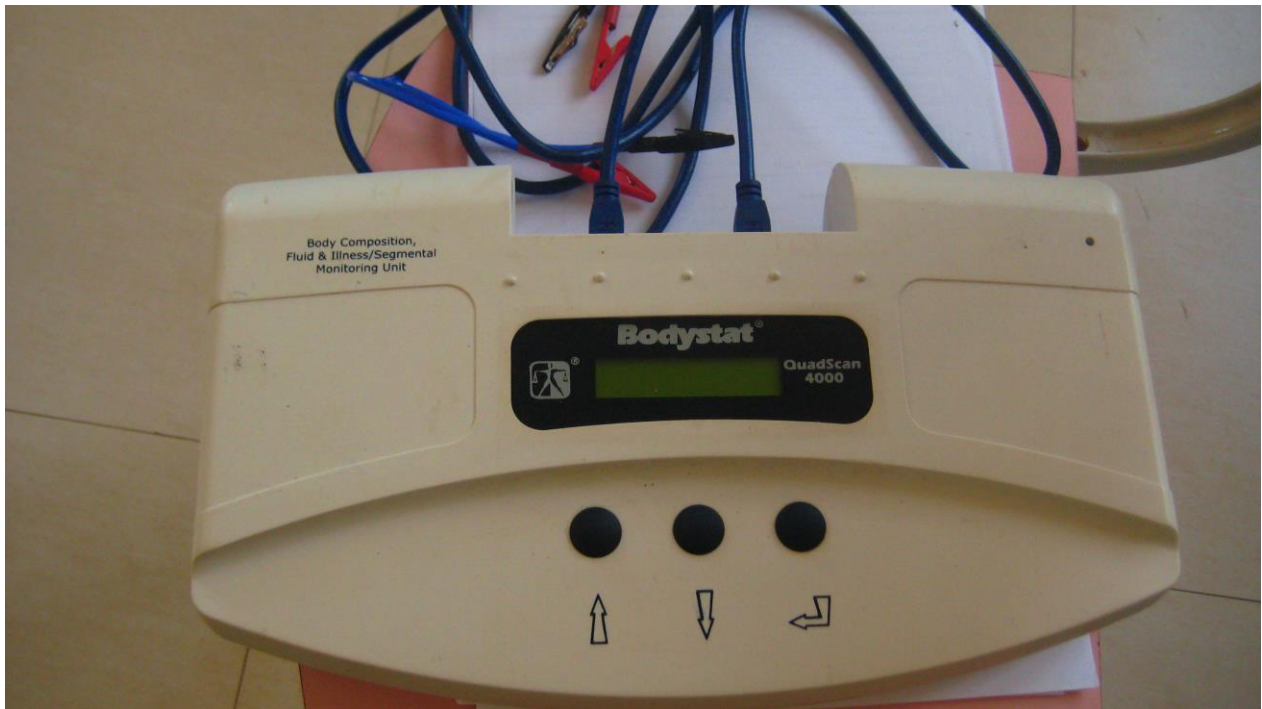
Figure 3.4 Bioelectrical impedance analyzer machine used for assessing bioelectrical impedance for research participants
