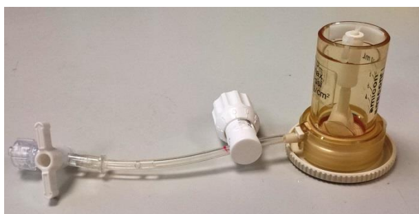
Figure 5-18 Manual pinch valve on the permeate line of stirred cell setup used for applying back pressure on the permeate line
