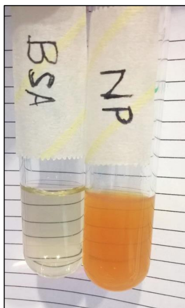
Figure 3-10 Turbid BSA nanoparticles preparation (labelled NP) obtained after precipitation of 1 mL of 100 g/L unmodified BSA solution (labelled BSA) using a mixture of methanol and ethanol as de-solvating agent (prepared using method C).
