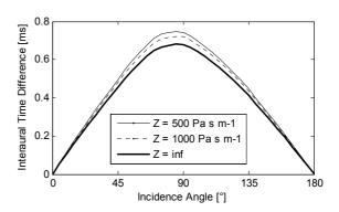
Figure 4. Change in interaural time difference with resistive impedance magnitude.
