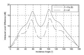
Figure 5. Change in ILD at 3000 Hz due to the approximate acoustic characteristics of hair.
