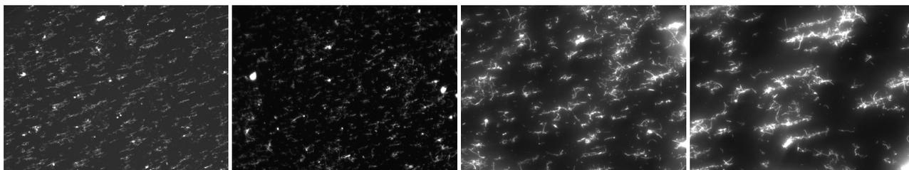
Figure 5: Fluorescent microscope images of fluorescent magnetic polystyrene nanowires aligned in an external magnetic field; from left magnification – x10, x20, x20 (increased lamp intensity), x40
