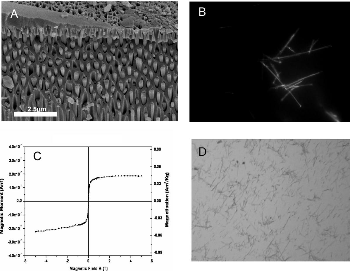
Figure 3: **A:** SEM image of fractured alumina membrane showing wires contained in pores; **B:** Confocal image of fluorescent silica nanowires; **C:** Magnetisation curve (VSM measurement) of maghemite loaded silica nanowires; **D:** optical microscope image of wires aligned in an external magnetic field.
