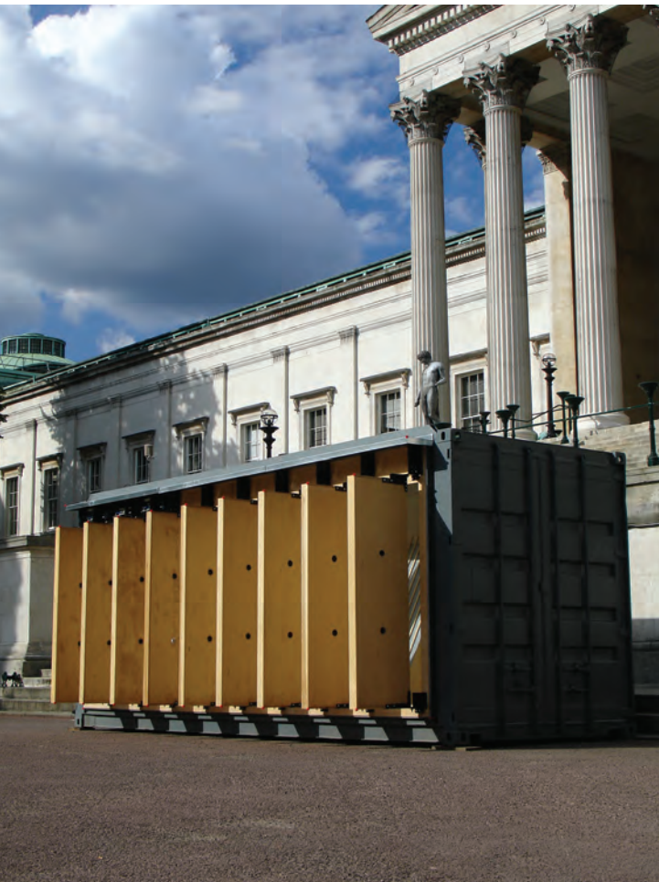
An actuator responds to different outdoor conditions by moving a façade's shutters
