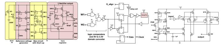
Fig. 3: Voltage regulator circuit (left); Clock and data recovery circuit (middle); Delay (T<sub>d</sub>) generator circuit in CDR (right);
