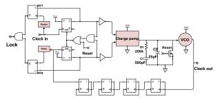
Fig. 4: Phased-locked loop and lock generation circuit.
