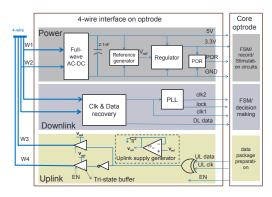
Fig. 2: Top-level system architecture for the 4-wire interface.
