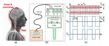
Fig. 1: System concept. (a) subcutaneous lead between implanted chest and head units; (b) Detail of 4-wire connectivity at each end of the lead; (c) how voltage waveforms on the 4-wire look like.
