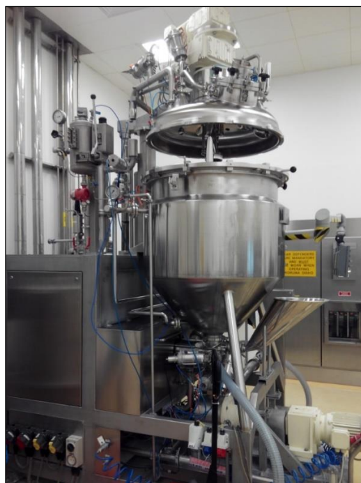
Figure 1. 4. Pilot plant scale mixer
