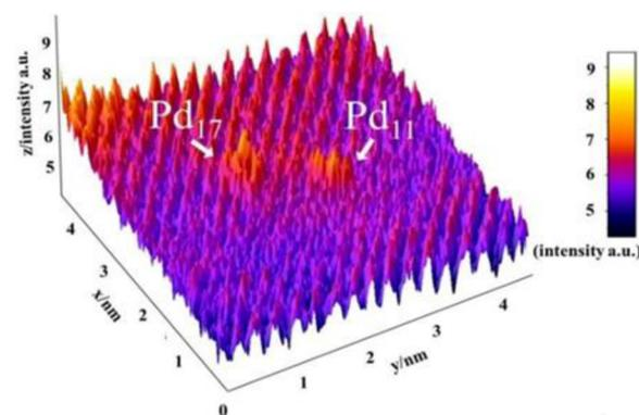
**Figure 2.** Processed HAADF STEM image of PdA1 showing Pd<sub>11</sub> and Pd<sub>17</sub> clusters.
