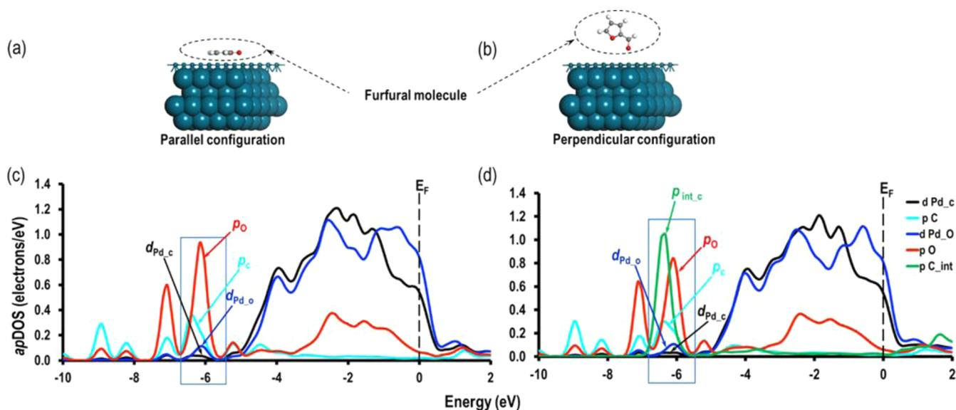
**Figure 8.** (a) Parallel and (b) perpendicular configurations of furfural on the Pd(111) surface. (c) *apDOS* for pristine Pd(111) and (d) *apDOS* for furfural on the PdC(111) surface. Black and blue lines represent the signatures for Pd d orbitals close to C and O atoms, respectively. Red, aqua, and green lines represent the p orbitals due to C, O, and interstitial C atoms, respectively.
