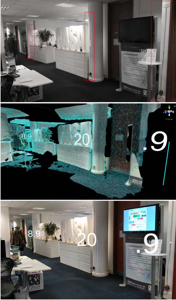
Fig. 2: Merging virtual and physical IoT. From top to bottom: actual environment, virtual reconstruction with sensor data readings incorporated, IoT data appended to physical objects. (Data overlaid to weather actuator light-strips which were developed by Steven Gray)
