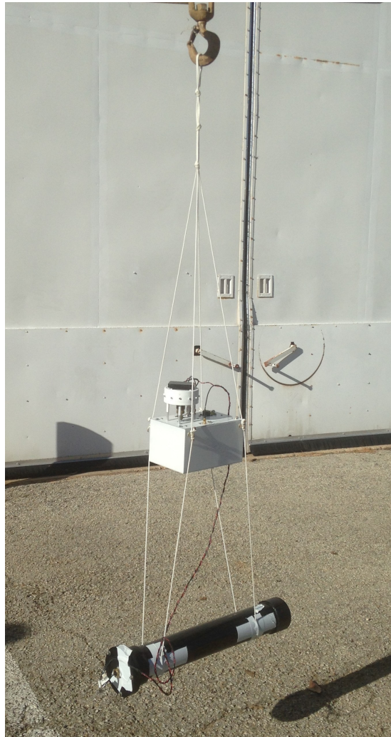
Figure 14: The hang test at CSBF, where all systems performed nominally, verifying payload-readiness for the Antarctic flight.
