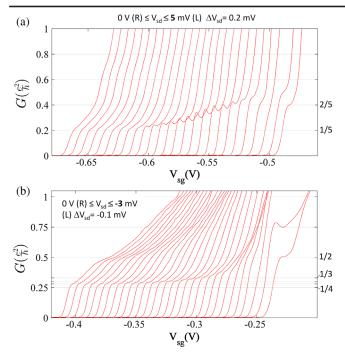
FIG. 4. Effect of dc source-drain bias on the fractional conductance. (a) The source-drain bias,  $V_{sd}$  was incremented from 0 (right, R) to 5 mV (left, L) in steps of 0.2 mV;  $\Delta V_{sg} = 955$  mV,  $V_{tg} = -0.36$  V (sample 1, cooldown 2). (b) Investigation of an Ohmic 1/2 structure;  $V_{sd}$  was incremented from 0 (R) to -3 mV (L) in steps of -0.1 mV;  $\Delta V_{sg} = 0$  mV,  $V_{tg} = -0.62$  V (sample 2, cooldown 3).
