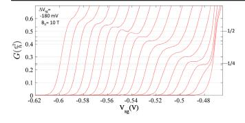
FIG. 2. Effect of variation of carrier concentration on the conductance in the presence of  $B_{II}$  (sample 2, cooldown 2). $V_{tg}$  was varied from -0.45 (left) to -0.62 V (right) in steps of -10 mV, at  $B_{II} = 10$  T;  $\Delta V_{sg} = -180$  mV.
