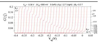
FIG. 3. Effect of variation of  $B_{II}$  on the fractional states (sample 1, cooldown 1).  $B_{II}$  was varied from 0 (left) to 12 T (right) in steps of 0.5 T;  $V_{tg} = -0.36$  V;  $\Delta V_{sg} = 800$  mV.
