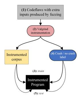
Fig. 2: Experimental setup for RQ1. Codeflaws is a augmented with additional inputs producing crashing and non-crashing executions (1). These are then instrumented with Valgrind (2). A neural network is trained on the instrumented executions (3) and crash / no crash labels (4). The performance of the NN classifier is then evaluated on a held out test set (5).
