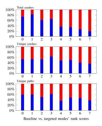
Fig. 7: Distribution of mean scores of baseline modes (blue, bottom part of bar) and targeted modes (red, top part of bar). The plots are of total crashes found, unique crashes found and paths found from top to bottom.
