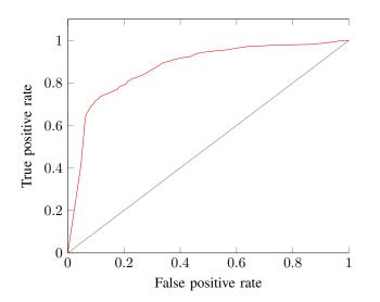
Fig. 5: The Receiver Operator Characteristic curve for the distribution in Fig. 4. The red curve represents the false positive *vs* true positive rate of crashing execution classification, corresponding to the red (RH peak) distribution in Fig. 4. The total AOC here is 0.887. The black diagonal line represents the indifference curve.
