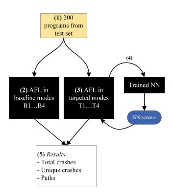
Fig. 3: Experimental setup for RQ 2. 200 programs are sampled from the test set (1). The programs are fuzzed in baselines modes (2) and modified targeted modes (3). Targeted modes query a trained NN for crash likelihood scores (4). The number of total crashes, unique crashes and discovered paths are recorded (5).
