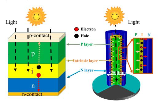
**Figure 3.** Illustration of the propagation path of photon and carriers in (**left**) thin-film solar cells and (**right**) NW solar cells.
