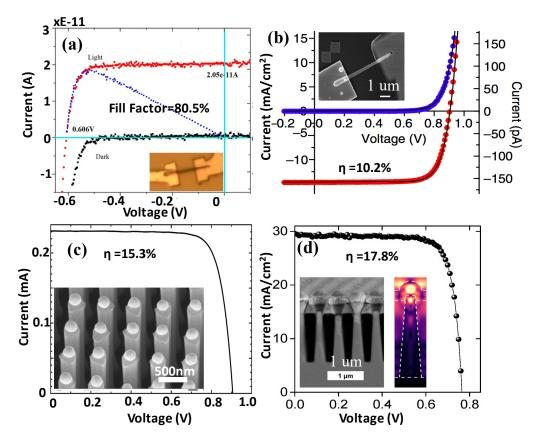
**Figure 5.** Dark/light current–voltage data and data of single (**a**) GaAs NW [91] and (**b**) GaAsP NW [109] solar cells. Current–voltage characteristics of (**c**) GaAs NW [92] and (**d**) InP NW [113] solar cells measured under 1 sun (AM1.5G) illumination. (**b**) Reprinted by permission from Springer Nature: Nature Communication [109], (Copyright) (2013). (**d**) Reprinted with permission from [113], Copyright (2016) American Chemical Society.
