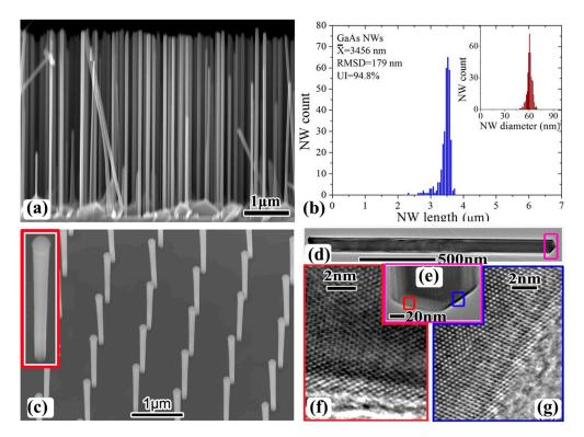
**Figure 1.** (**a**) Sideview of GaAs nanowires (NWs) on unpatterned Si substrate. (**b**) Length and diameter summation histogram of NWs in (**a**) [32]. (**c**) GaAsP NWs on patterned Si substrate [36]. (**d**–**g**) One defect-free GaAsP NW [37].
