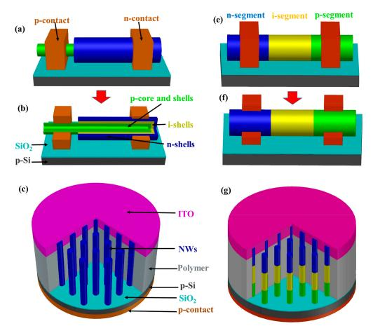
**Figure 4.** Illustration of single (**a**,**b**,**e**,**f**) and large-area (**c**,**g**) solar cells with radial (**a**–**c**) and axial (**e**–**g**) p–i–n junctions.
