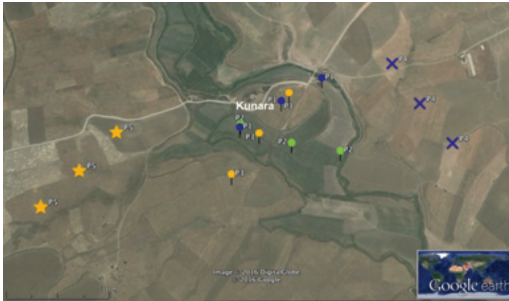
Fig. 28: Google Earth image showing the ERT profiles (marked as points) near Kunara. The points are marked for the profile numbers and indicate the ends and middle location of the 345 m transects © Mission archéologique du Peramagron.
