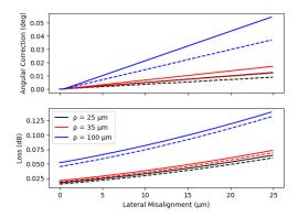
Fig. 9. Required angular correction to compensate for a given lateral misalignment at the collimator, for  $\rho=25\,\mu m,\,35\,\mu m,\,100\,\mu m.$  Dashed lines indicate a MFD of  $12\,\mu m,$  solid lines indicate a MFD of  $8\,\mu m.$  The maximum actuator angle is 10 degrees and the loss is wavelength independent.
