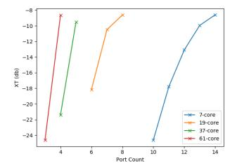
Fig. 16. Total crosstalk (XT) after 1 km on the central core of a 7/19/37/61 core hexagonal homogeneous TA-MCF for the minimum value of mode coupling coefficient at which single mode operation is maintained, with a fixed pitch of  $25 \,\mu\text{m}$ , operating at a wavelength of 1550 nm. Port counts are calculated assuming that the optimal  $f_1/f_2$  values are used for each design.
