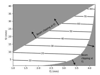
Fig. 4.  $z_2$ (mm) as a function of  $f_1$  and  $f_2$ . The maximum value of  $z_2$  occurs at the maximum possible values of  $f_1$  and  $f_2$  which are in turn restricted by the beam clipping at their respective lenses.
