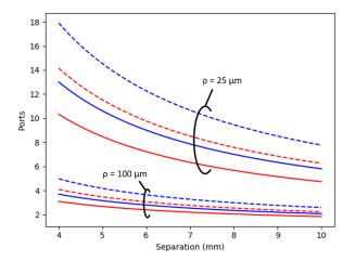
Fig. 6. Maximum number of ports in a single dimension as a function of the port separation, with maximum actuator angle set to 10 degrees. Dashed lines indicate a MFD of  $12\,\mu m$ , solid lines indicate a MFD of  $8\,\mu m$ . Red lines are wavelength of 1620 nm, blue lines are 1260 nm.  $\rho$  is the distance from the outer most core to the fiber center.
