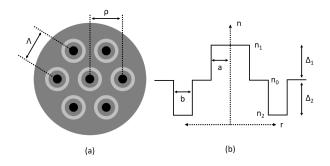
Fig. 11. (a) 7 core hexagonal TA-MCF, with core pitch,  $\Lambda$ , and distance from the outer most core to the fiber center,  $\rho$ . (b) Refractive index profile of a trench assisted core,  $n_0$  is the cladding refractive index, with the core and trench index raised and lowered to  $n_1$  and  $n_2$  respectively.
