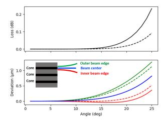
Fig. 7. Deviation of beam center and  $1/e^2$  edges versus actuator angle with corresponding estimated total loss from mode field diameter mismatch and lateral displacement. Dashed lines indicate a MFD of  $12\,\mu m$ , solid lines indicate a MFD of  $8\,\mu m$ . Red lines represent the edge of the beam closest to the fiber center, green the outer edge and blue the center of the beam. The  $f_1/f_2$  values are optimized for each angle. The deviation and loss is wavelength independent.
