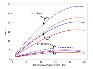
Fig. 5. Maximum number of ports in a single dimension as a function of the maximum actuator angle, with port spacing of 4mm. The  $f_1/f_2$  values are optimized for each angle. Dashed lines indicate a MFD of  $12 \, \mu m$ , solid lines indicate a MFD of  $8 \, \mu m$ . Red lines are wavelength of  $1620 \, nm$ , blue lines are  $1260 \, nm$ .  $\rho$  is the distance from the outer most core to the fiber center.
