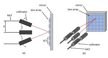
Fig. 1. (a) A one dimensional slice of the switch configuration with the overall structure shown in (b). Fiber collimators are steered by piezo actuators to pass through the center of the lenses within the array and imaged onto the exit fiber end face. Example beam paths are shown in red.
