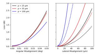
Fig. 8. Estimated total losses across all cores resulting from both angular and lateral misalignment between the collimator and lens array, for  $\rho=25\,\mu m,\,35\,\mu m,\,100\,\mu m.$  Dashed lines indicate a MFD of  $12\,\mu m,$  solid lines indicate a MFD of  $8\,\mu m.$  The maximum actuator angle is 10 degrees and the loss is wavelength independent.
