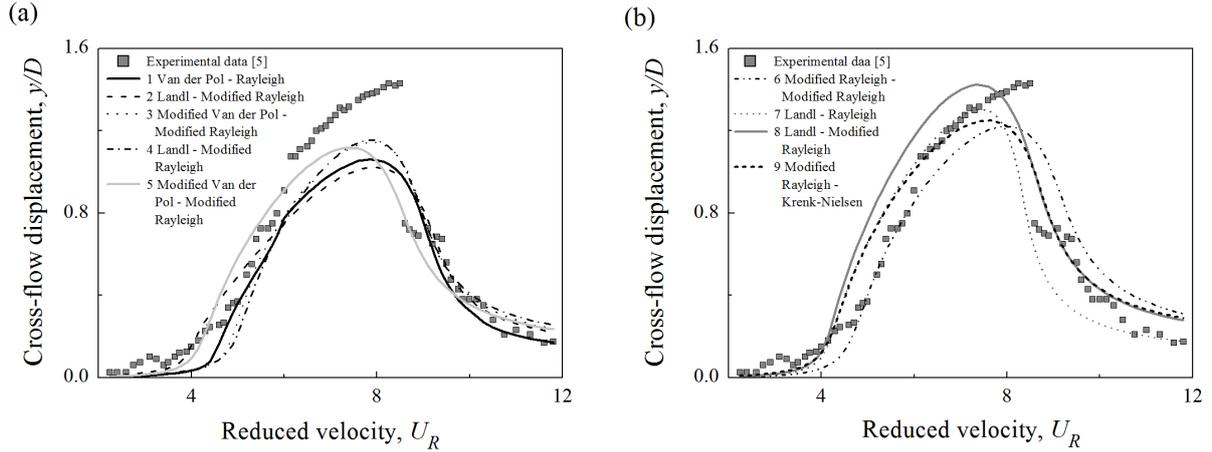
**Figure 11:** Experimental data by Blevins and Coughran [5] for mass ratio of 2.57 against displacement amplitudes predicted by the model variations of Library 2 from Table 8: (a) cross-flow displacement amplitudes predicted by Options from 1 to 5; (b) cross-flow displacement amplitudes predicted by Options from 6 to 9.
