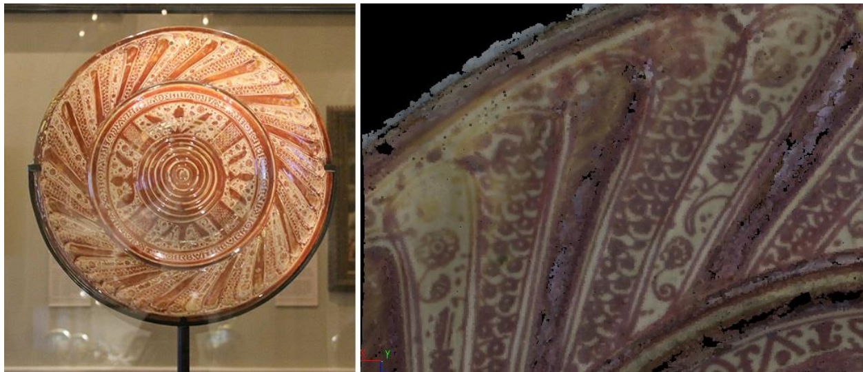
Fig. 1: L-R Photo of Lustreware bowl showing its extreme specular 4 ; detail of the unprocessed 3D model of the bowl showing noise and artefacts caused by the specular highlights (Photo: Lustred ceramic dish. Probably Valencia,
