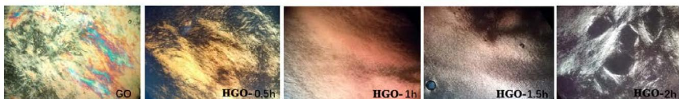
**Figure S2** POM images of GO and HGO with different etching time. As the etching time increasing, the POM image of HGO exhibited less colorful textile.
