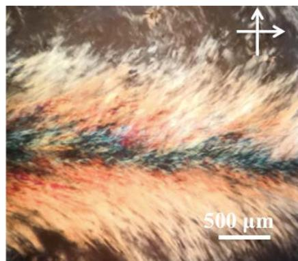
**Figure S3** POM image of the mixture of the holey graphene oxide and Vitamin C
