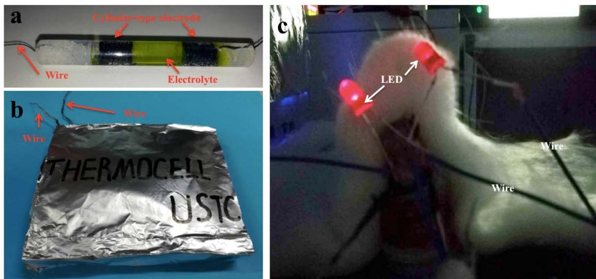
**Figure S14** Photographs of single cryo-thermocell (a), thermocell device (b, 15 in series) and the LED beads (c) were lighted by the thermocell device.
