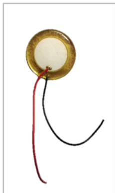
Figure 27 Picture of Microphone 3, a ceramic piezoelectric transducer, and a circuit diagram of the preamplifier used
