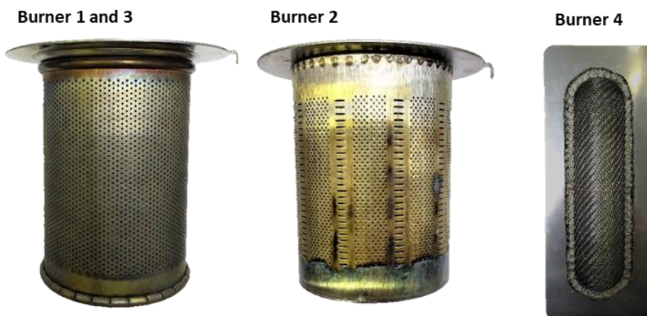
Figure 26 Pictures of Burner 1, 2 and 4 used in Boilers 1 and 2
